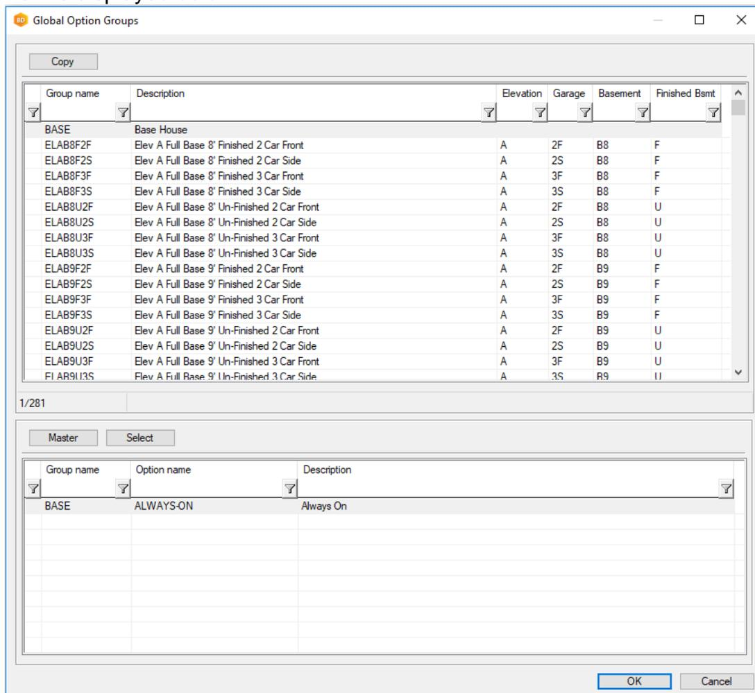
The option group database should always include the **BASE** option group, which is the base model of the building.
