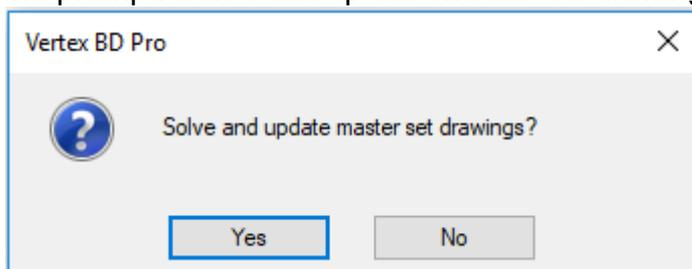
2 Select **Yes** in the message box. The program solves the options and creates the selected drawings. The program creates a subfolder in the project's MS folder according to the name of the option group. The drawings will be saved in this folder. The solved model remains active.
